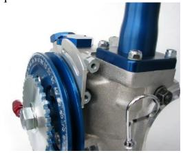
4. Install extension bracket, leave bolts loose enough to allow the extension to slide.
