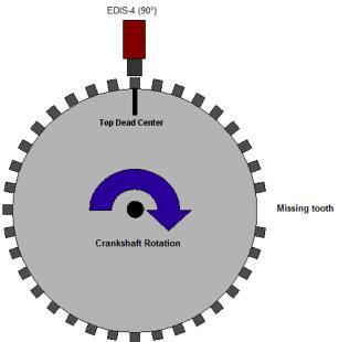
6. Use provided shims if necessary to shim sensor at least .020" from trigger wheel. Tighten everything down making sure the sensor is **centered over** the 9<sup>th</sup> tooth.
