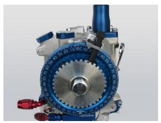
5. Install Crank sensor into extension bracket. <u>Line up the</u> sensor over the 9<sup>th</sup> tooth counter clockwise from the missing tooth on the trigger wheel.
